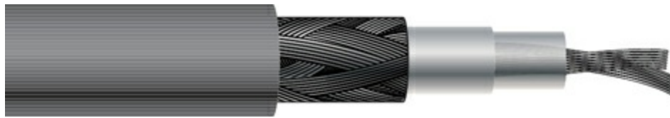
Figure 5-3 Coaxial Cable
