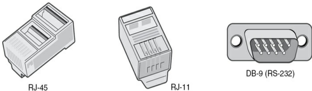
Figure 5-7 Twisted-Pair Cable Connectors
