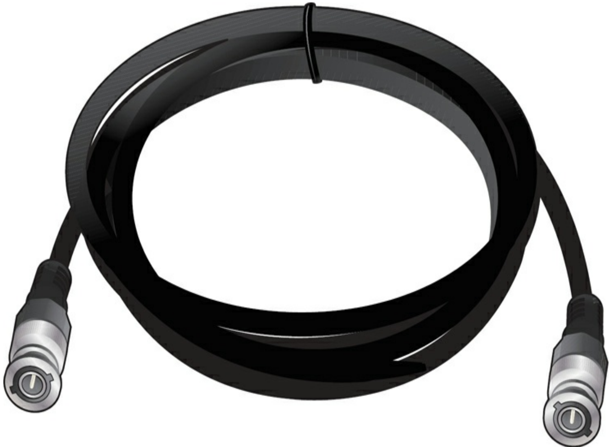
Figure 5-13 Coaxial Cable Used for 10BASE2
